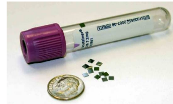
2 mm X 2 mm tags include antenna
